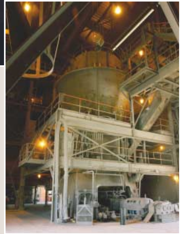
The roller mill uses recycled kiln gases for drying the limestone and clay during this stage of the grinding process.
