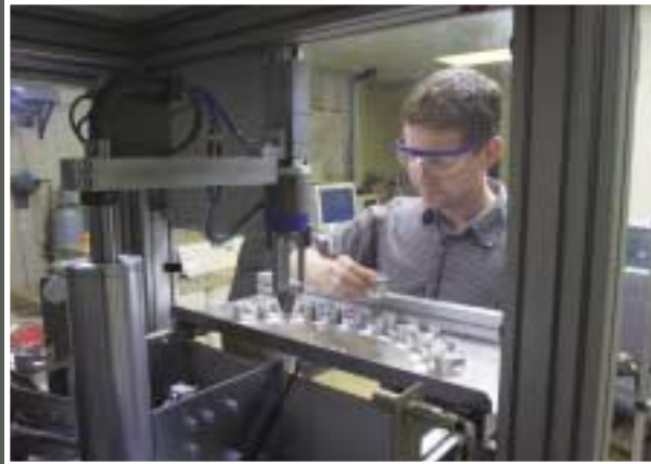
A state-of-the-art lab is used to analyze the raw material, maintain quality control and formulate special products. Lab Technician, Mike Stanzel begins fusing cement samples before x-ray analysis.
