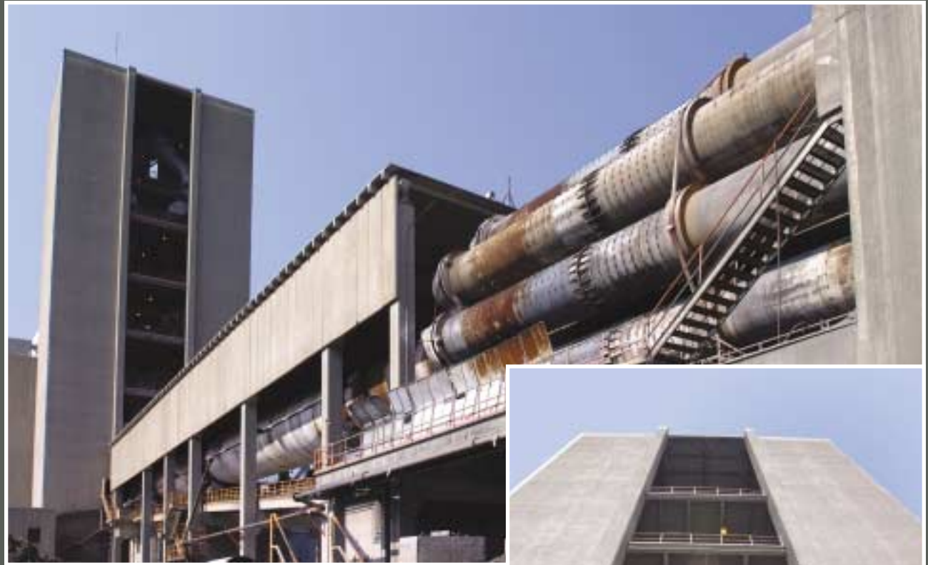
The 75m long kiln rotates twice a minute as the raw material rolls and slides along its length.
