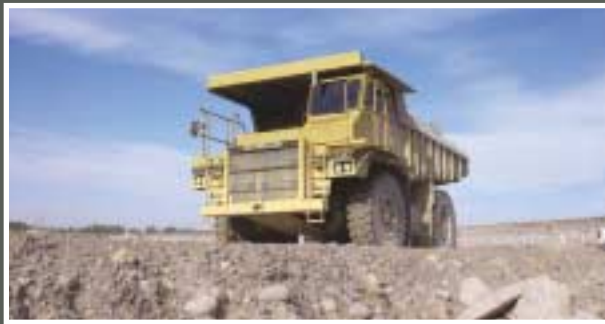
Hardworking 40 tonne quarry trucks transfer shot rock from the face to the primary crusher within the quarry.
